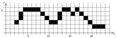
Chain code: ne-n-ne-e-e-e-se-se-se-e-ne-n-ne-e-se-ne-se-se-se-e-e
